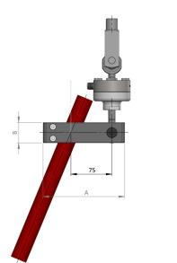
Clamps for fatigue tests with vertical forces ISO 4210-6 parte: 4.5 EN 15194 parte: 4.3.7.6
